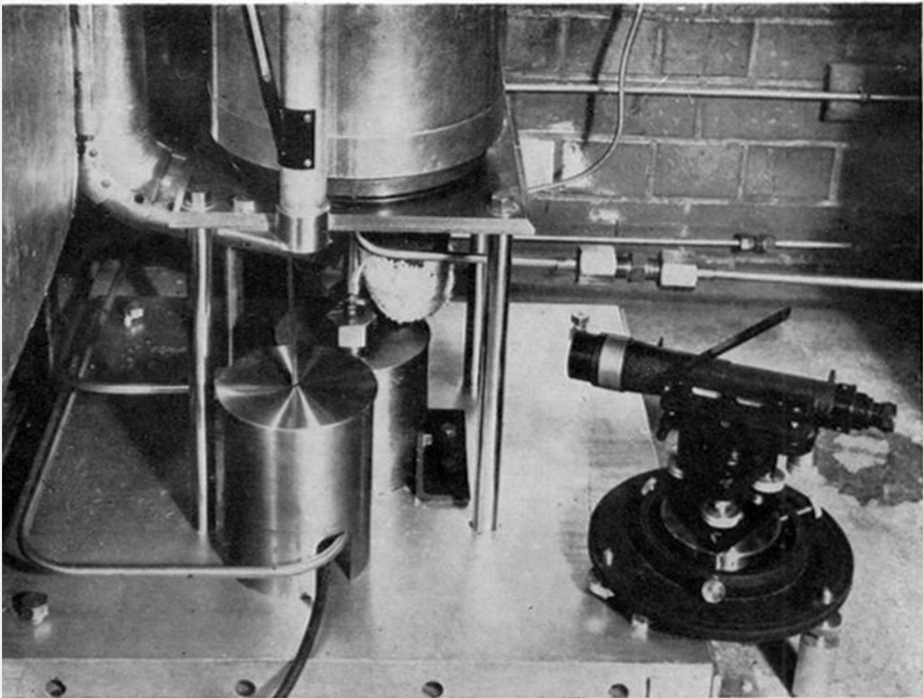
FIGURE 6. Photograph of the base of the mercury column with the lagging removed.
